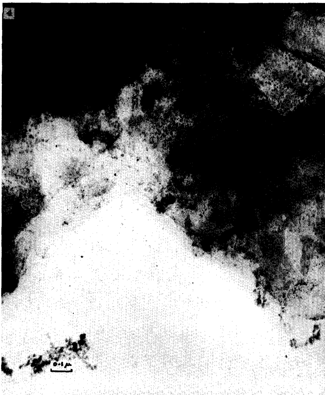
Fig. 4. Catalyst A-2 after reaction showing loss of decoration.
