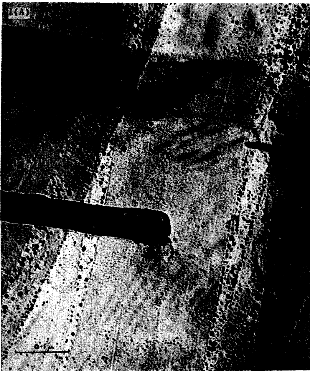
FIG. 1. (a) Decorated catalyst A (from \text{PdCl}_2 ); (b) decorated catalyst B (evaporated Pd).
