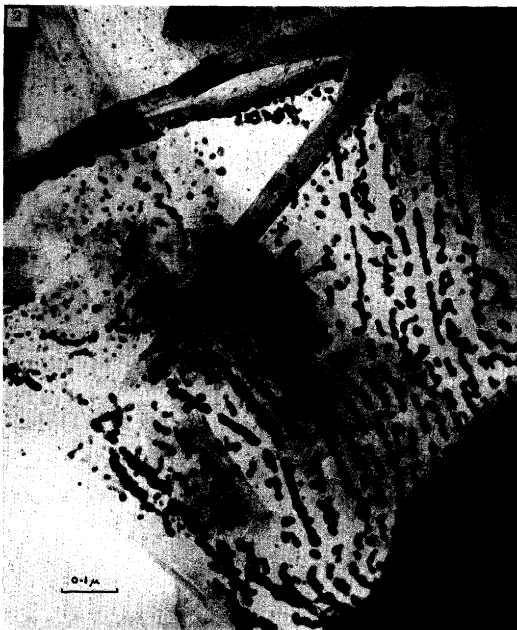
Fig. 2. Catalyst B-2 showing nucleation after reaction at 43°C.
